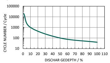
Charging Condition : CV(3.4V, 200 $\Omega$ , 48H) Discharging Condition : CR(30k $\Omega$ , 2.5V Cut-off)
